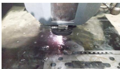
Fig 3.1 Machining process using EDM
